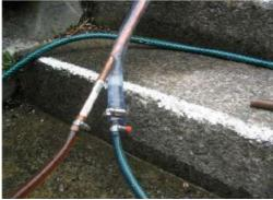
The picture above shows the bottom part of my pre cooler. At the time of the picture, there was a brew going through the silicone hose that connects the pre cooler with the main cooling coil.
