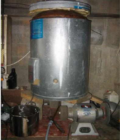
Under the boiler you can see a copper pipe connecting to a hot water rated plastic water pipe going to the cooler. What you can not see is the valve between the boiler and the copper pipe. This valve will ensure your brew is not lost.
