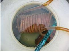
The picture above shows the main cooling coil submerged in cold water. The silicone hoses are transparent so you can clearly see what is going on and ensure that your brew is clear with no hops and/or proteins. You can also see a garden hose constantly pushing in cold water to the bottom whereas hot water is overflowing at the top. This cooling arrangement brings down the temperature to about 25-30C. Perfect for the yeast!
